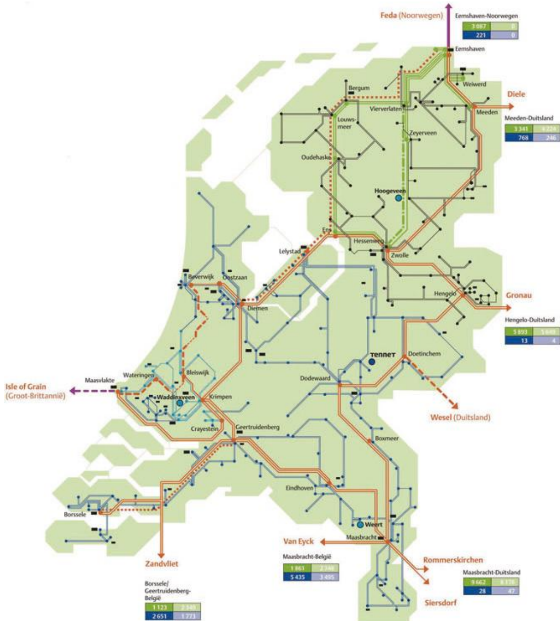
Figure 21: High voltage network in the Netherlands
