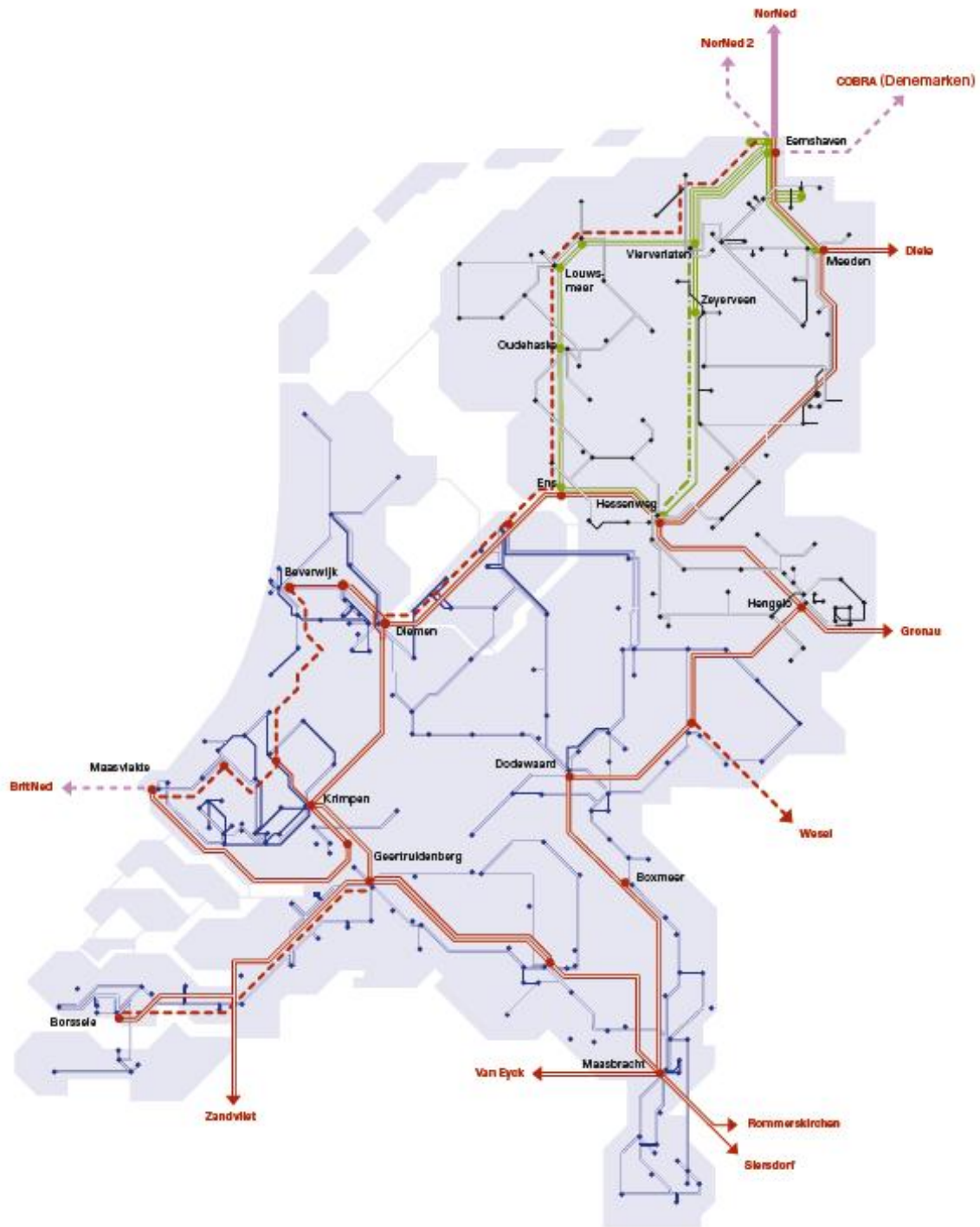
Figure 20: High voltage network in the Netherlands
